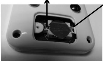
④ For the battery change, please gently pry out the battery with a thin blade.
