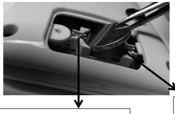
Make sure the right side battery connector is on top of the battery.
