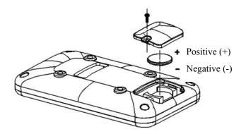
③ Install a new CR2032 battery by tilting the battery slightly to its side and slide it in. (positive (+) at upper side and negative (-) at down side)
